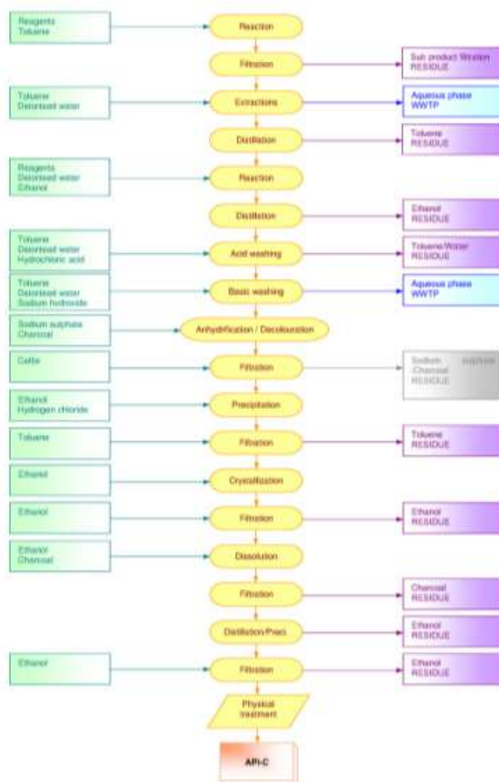
Figure 7: Example API production flow diagram
